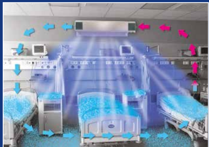
Process of the air treatment with the use of internal and external UV-C tube (air and surfaces)
