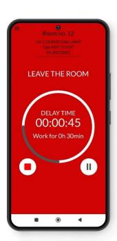
The NBV 8x36 P BT and NBV 8x75 P BT lamps are equipped with a programmable switch module controlled by the NBV App via a smartphone or tablet with Android (Bluetooth).
